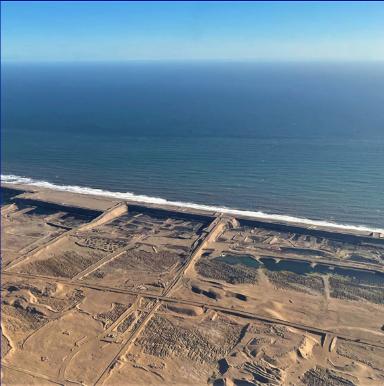
Aerial view of submerged beach mining activities in Namibia, where diamondiferous gravel is being mined behind a sea wall approximately 30m below sea level.
