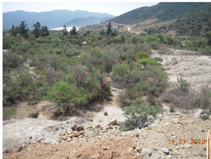
Figure 5 – Tailings flow deposits from the El Cobre dam failures (foreground)
